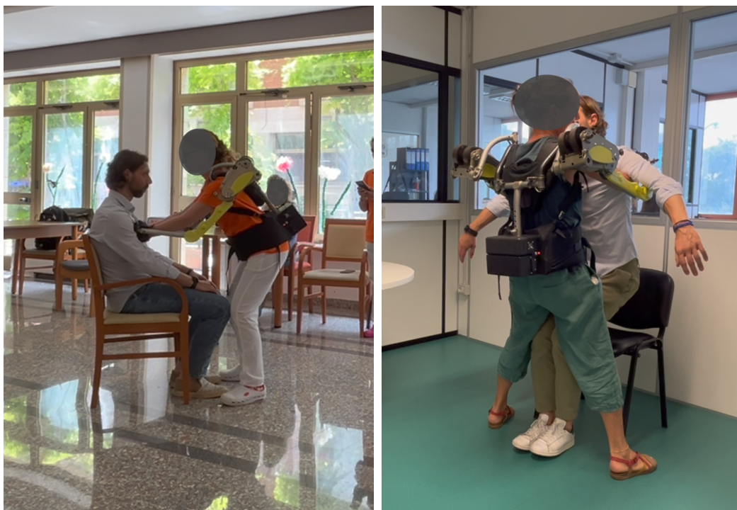
Figure 1. Simulated patient handling tests conducted by healthcare workers (OSS) while wearing the passive exoskeleton in a controlled real-world environment. Task: lifting and moving a patient from one seat to another.
