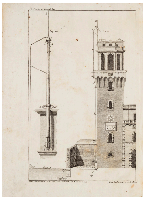
Figure 3: Lightning rod on the Padua Observatory, installed by Giuseppe Toaldo in 1773. Illustrated in a 1774 engraving by Franco Castellani and Giuseppe Zulian. Credit: Deutsches Museum.
