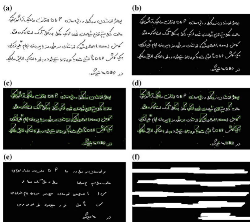
Fig. 6 - Application of erosion and dilation techniques (a, b, c, d, e) followed by Gaussian blur (f) to extract lines (Bugeja 2020)
