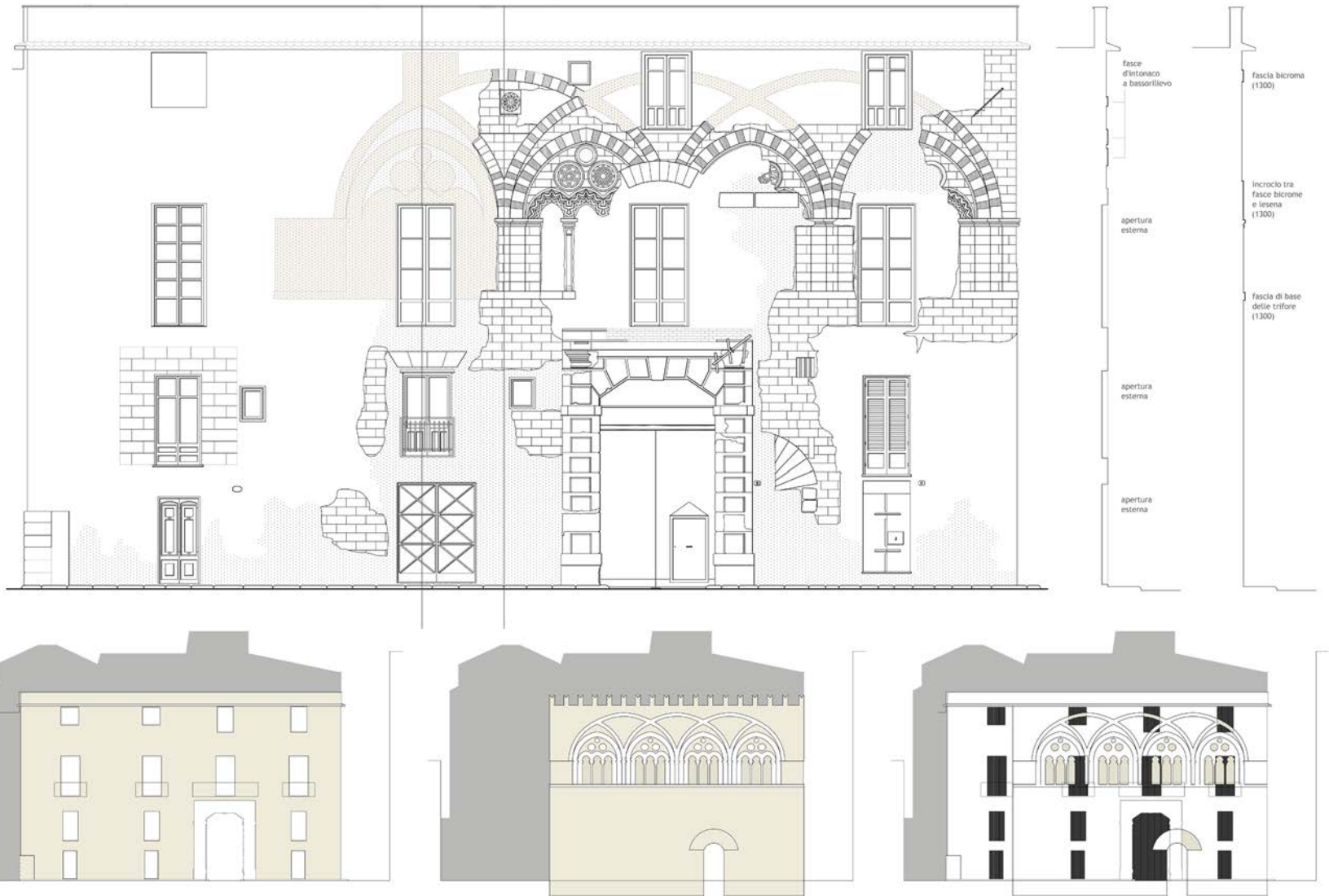
Fig. 12: Proposal for the restoration of Palazzo Cefalà in Palermo: preservation of all the architectural elements that can be attributed to each phase of the transformation of the building and critical reintegration of the gaps in the plaster. Below: graphic overlay between the nineteenth-century facade and the front view of the Chiaramonte tower-house (by the author).
