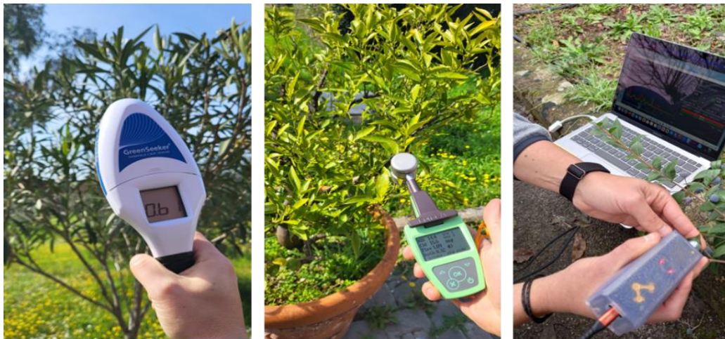
Fig.2 Field-monitoring of plant physiological responses is conducted using portable optical instruments: Greenseeker (left), Dualex (center), and Raman spectrometer (right)
